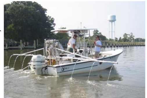
Mechanical seed broadcast machine spraying eelgrass seeds at a bay grass restoration site
