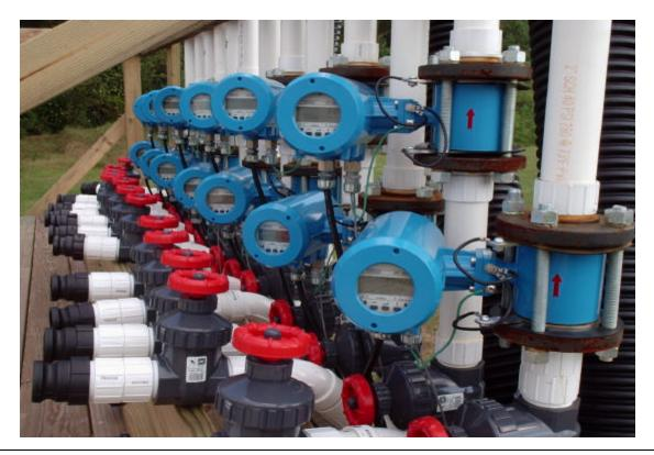
The flowmeters selected for use in the study were the Kronhe Model IFS 1000 Wafer Style Flowmeter with the Model IFC 090 Converter. This type of flowmeter was selected for the following reasons:
