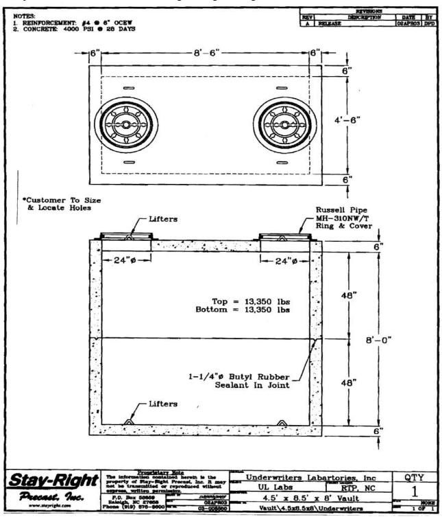
The underground storage tank was constructed of reinforced concrete and had the following internal dimensions:
