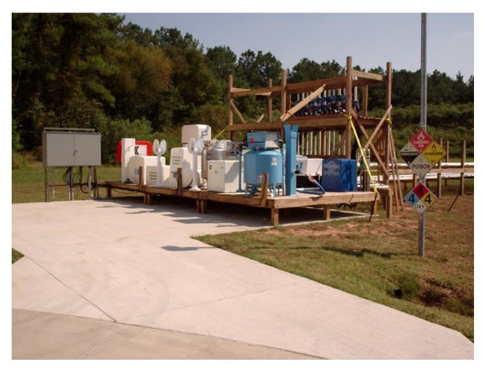
The units were mounted on a simulated dock structure to closely match the actual mounting of the units in a marina. The dock structure was supported on a concrete pad.
