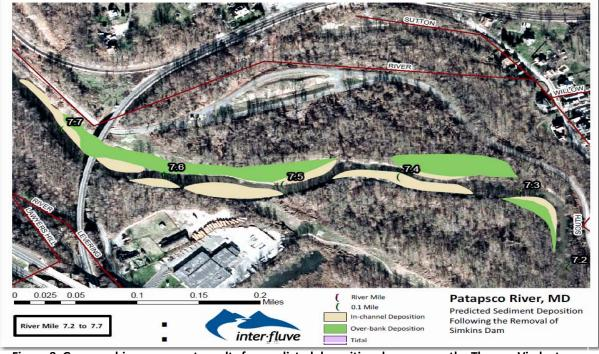
Figure 8. Geomorphic assessment results for predicted depositional areas near the Thomas Viaduct2012 Inter-Fluve, Inc.Bloede Dam Alternatives Analysis
